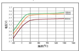
3. Capacity VS Temperature(cut off at 2.0V)
