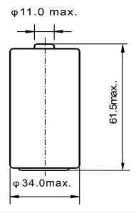
Size unit:mm (GB1804-m if tolerance is not specified)
